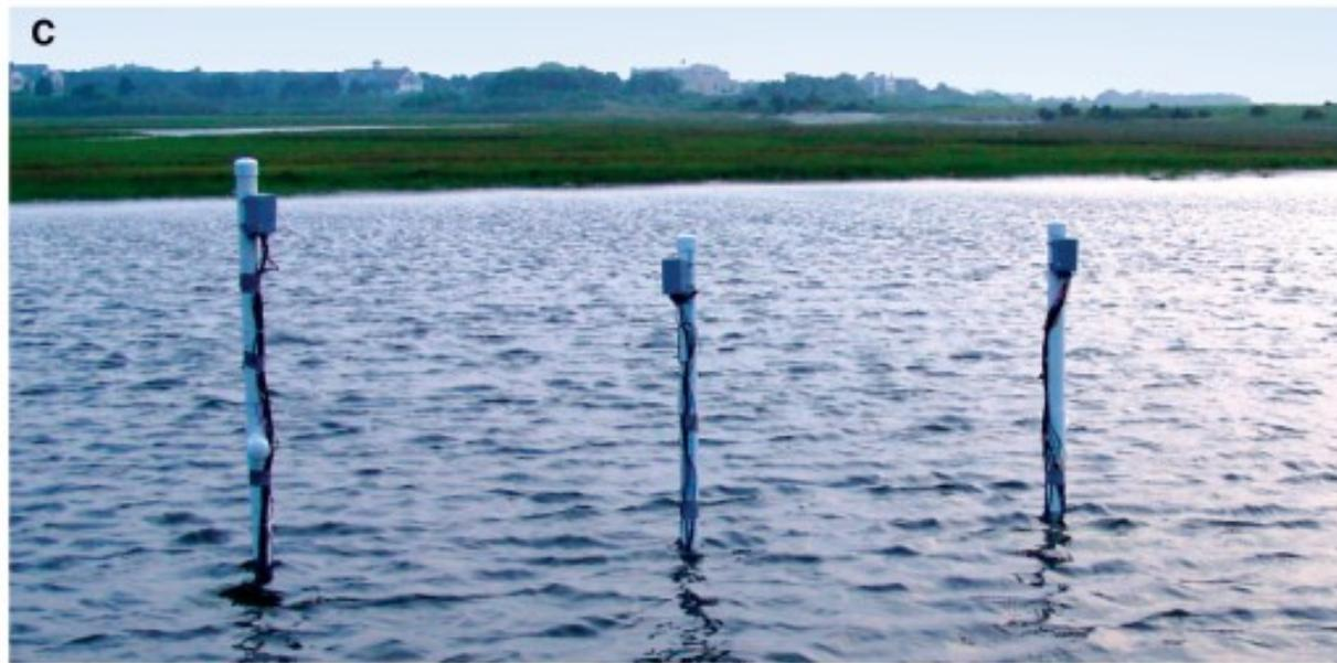
Sediment fuel cell. (A) Prior to deployment in salt marsh sediments on Nantucket Island, Mass. (B) Diagram of sediment fuel cell reactions. (C) Deployed sediment fuel cells. (Photos courtesy of Kelly Nevin, University of Massachusetts-Amherst.)
